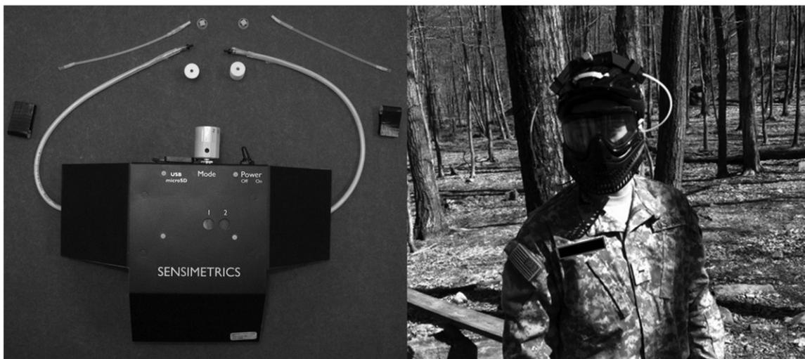
**Figure 2.** Hearing loss simulator (HL Sim) shown in close-up (left) and when mounted on top of a participant's helmet/mask (right). The knob on the front of the HL Sim was used to select between the preloaded hearing loss simulation profiles. Note the wooded and hilly terrain behind the soldier, which is a view of the playing area near the centre staging zone at the US Military Academy site.
